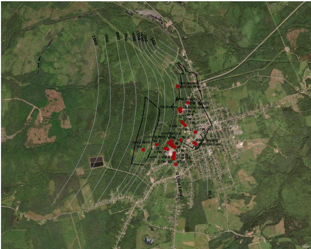
Figure E4: Satellite image of Springhill showing geothermal borehole locations, the No. 6 coal seam workings and the No. 6 coal seam contour elevations.
