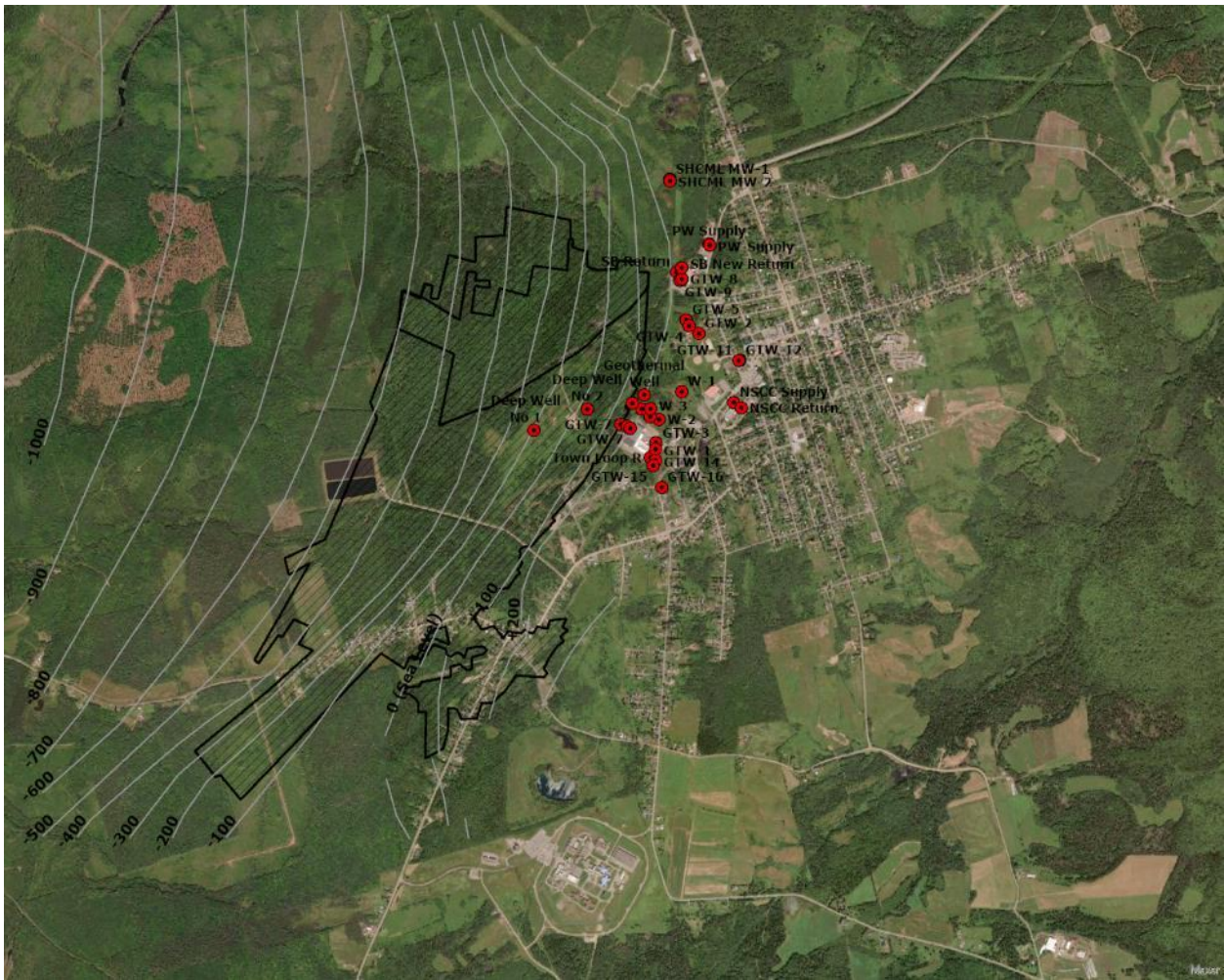
Figure E3: Satellite image of Springhill showing geothermal borehole locations, the No. 3 coal seam workings and the No. 3 coal seam contour elevations.
