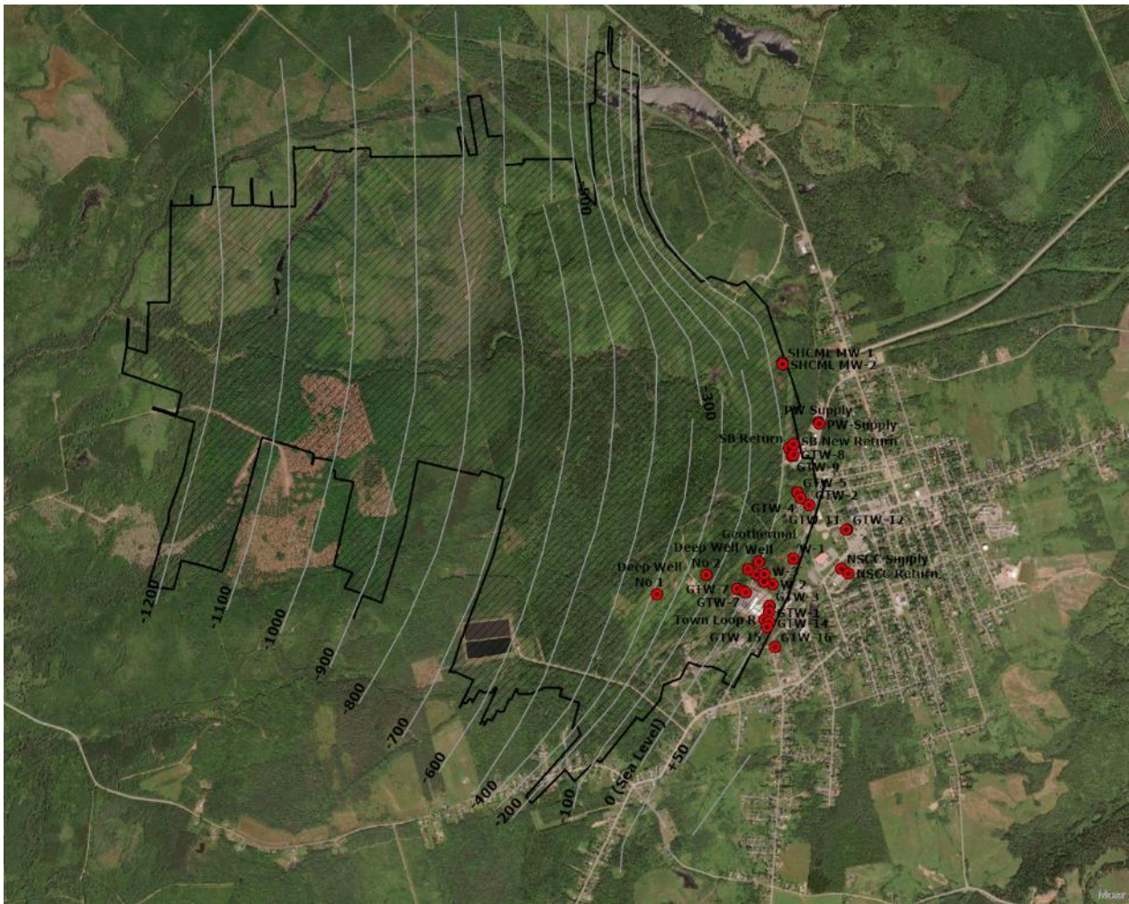
Figure E2: Satellite image of Springhill showing geothermal borehole locations, the No. 2 coal seam workings and the No. 2 coal seam contour elevations.
